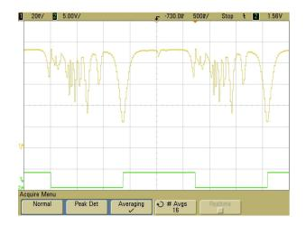
Figure 3. Spectrum analyzer: measured spectrum of a -10 dBm 100 MHz sinusoid. Horizontal axis is RF input frequency. Upper trace vertical axis is logarithmic video output voltage, at 20 mV/div. Bottom trace: falling edge indicates frequency synthesizer transition from 200 MHz to 1.56 MHz, rising edge indicates 100 MHz. Large dip in upper trace indicates strong 100 MHz RF input signal. Output is inverted, where lower voltages indicate stronger signals.
