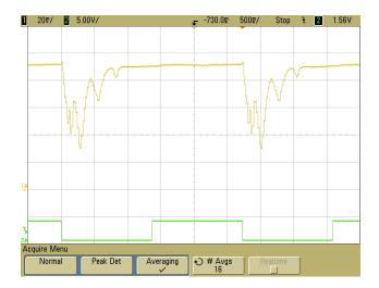
Figure 6. Spectrum analyzer: measured spectrum of a 20 MHz, -10 dBm sinusoid. Horizontal axis is RF input frequency. Upper trace vertical axis is logarithmic video output voltage, at 20 mV/div. Bottom trace: falling edge indicates frequency synthesizer transition from 200 MHz to 1.56 MHz, rising edge indicates 100 MHz. Large dip in upper trace indicates strong 20 MHz RF input signal. Output is inverted, where lower voltages indicate stronger signals.
