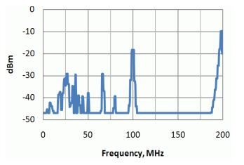
Fig. 9 Spectrum analyzer: measured spectrum of 200 MHz -10 dBm sinusoid. Horizontal axis is RF input frequency, vertical axis is logarithmic video output converted to equivalent power level in dBm.
