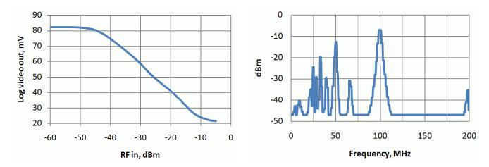
Figure 4. Spectrum Analyzer response to a 100 MHz RF input signal Horizontal axis is RF input power; vertical axis is logarithmic video output.
