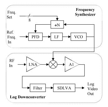
Figure 1. Block diagram of the proposed single chip Spectrum Analyzer with frequency synthesized tuning. Spectrum Analyzer and Frequency Synthesizer blocks are marked for clarity.
