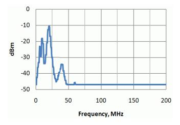
Figure 7. Spectrum analyzer: measured spectrum of 20 MHz -10 dBm sinusoid. Horizontal axis is RF input frequency, vertical axis is logarithmic video output converted to equivalent power level in dBm.
