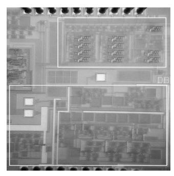
Figure 2. Photograph of single-chip spectrum analyzer; upper box surrounds frequency synthesizer, lower box surrounds remainder of spectrum analyzer.
