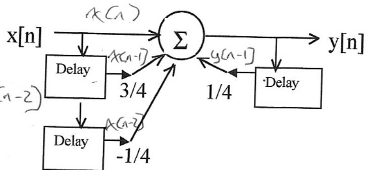
26. In the difference equation for the block diagram above, the weight A is A=
