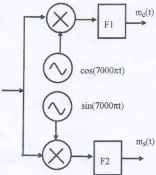
In the system above with input  $f(t)$  and with outputs  $m_c(t)$  and  $m_s(t)$ , filters F1 and F2 are ideal lowpass filters with bandwidth 200 Hz.
