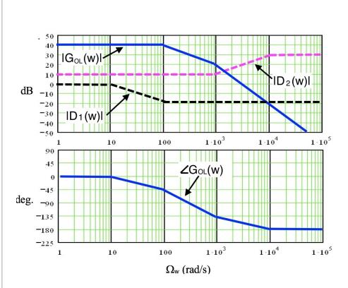
For the w-transforms shown above, the Bode plots for phase of the two compensators are not shown (you may assume the phases are the correct Bode plot phases for lag, lag-lead, PID, or lag compensators). For **uncompensated** open-loop gain  $G_{OL}(w)$  shown above, using Bode plot analysis the gain margin to within +/-3 dB is
