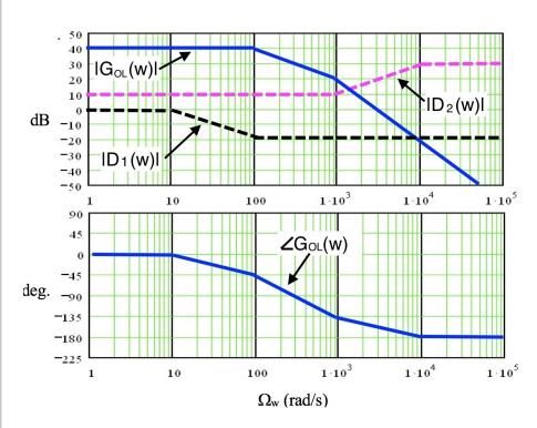
For the w-transforms shown above, the Bode plots for phase of the two compensators are not shown (you may assume the phases are the correct Bode plot phases for lag, lag-lead, PID, or lag compensators). For open-loop gain  $G_{OL}(w)$ , comparing the bandwidth using the two compensators, the unity-gain bandwidth of  $G_{OL}(w)D_1(w)$  is larger than  $G_{OL}(w)D_2(w)$ .
