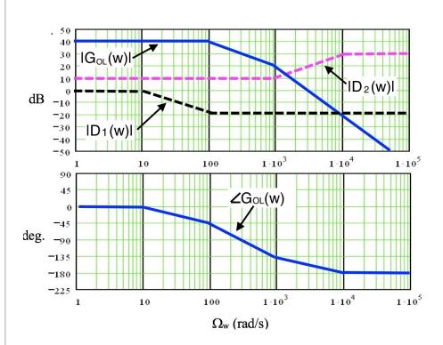
For the w-transforms shown above, the Bode plots for phase of the two compensators are not shown (you may assume the phases are the correct Bode plot phases for lag, lag-lead, PID, or lag compensators). For open-loop gain  $G_{OL}(w)$  combined with compensator  $D_1(w)$  shown above, the gain margin of  $G_{OL}(w)D_1(w)$  to within +/-4 dB is
